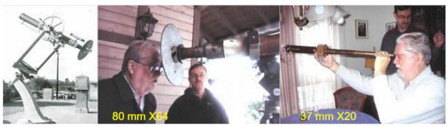
**Fig. 4.** Left: the 80 mm Fraunhofer refractor used since 1855 by Wolf and successors. Center: the same telescope in use today by Thomas Friedli (person at right). Right: the 37 mm portable telescope used by Wolf since the mid-1860 s.
