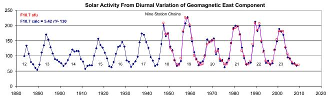
Fig. 7. 10.7 Flux correlation with the range, rY, of the diurnal variation of East Component.
